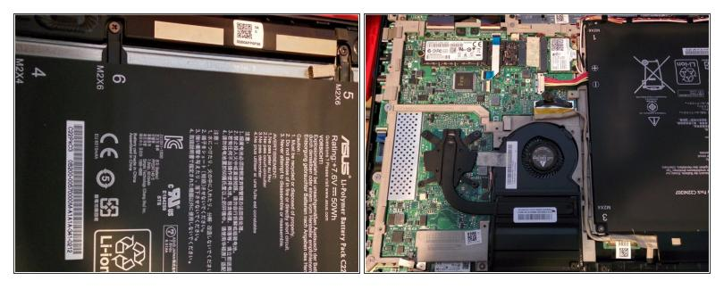
• The battery is attached via 6 screws. They are clearly marked with location and screw size.
