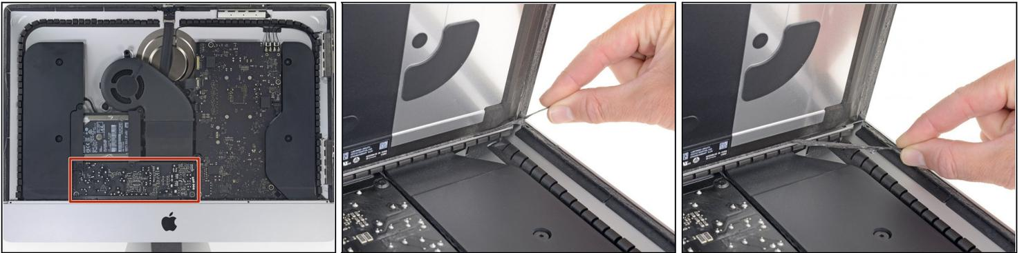
**⚠** Be very careful not to touch the capacitor leads or any exposed solder joints on the back of the power supply (boxed in red).
