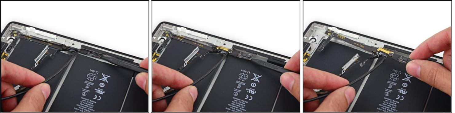
ⓘ To remove the upper component board you will be pulling gently on its cable while lifting it up enough to clear the battery, but not high enough to scrape against the rear case. Go slowly and carefully.
