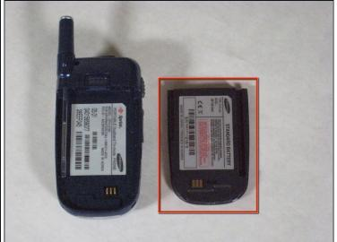
• Push open the latch and remove the battery.
