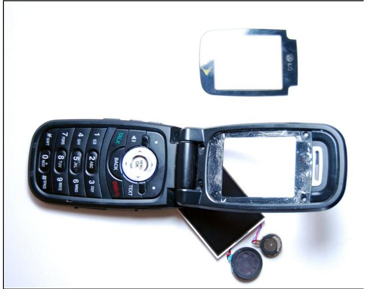
**⚠ Apply even amounts of force upon removing screen, otherwise cracking may occur.**
