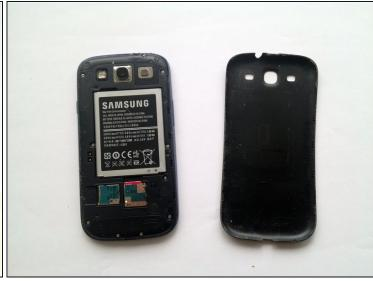
With a plastic opening tool, pry open the back case. It will come out very easily.
