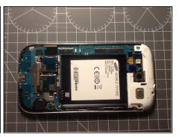
• Use the spudger to gently pry the display data cable from the motherboard.
