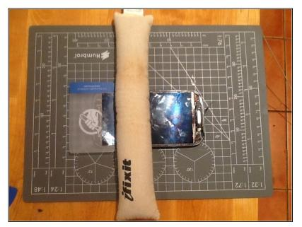
As you work you will want to reheat the iOpener and put it back on the display to melt the adhesive further down the screen
