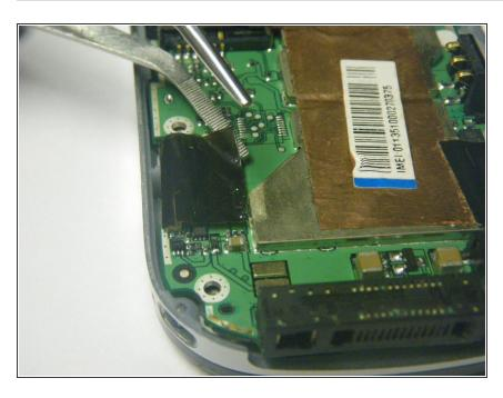
Carefully peel back the tape holding the speaker (left) and keyboard (right) connection tabs in place.
