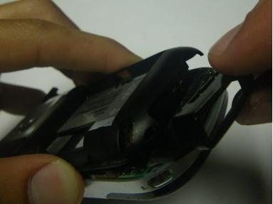
Remove the small plastic insert at the bottom of the phone.
