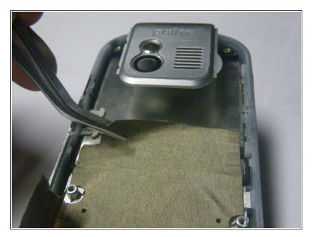
Slowly peel off the protective lining that is on the screen and keyboard.
