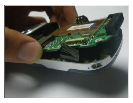
Separate the logic board from the case by lifting and pulling out the bottom.
