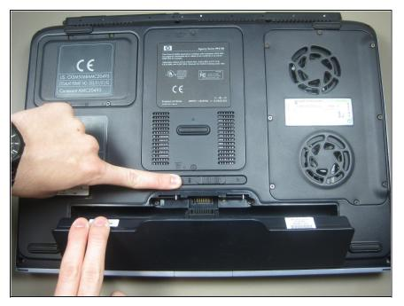
Slide the battery release switch to the right while simultaneously lifting up the battery.
