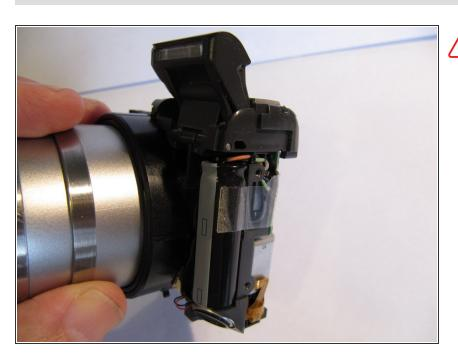
Note the large cylindrical flash capacitor which could still hold a dangerous high voltage charge if the camera has been switched on recently. Do not remove protective insulation on this and surrounding components unless you know how to discharge the capacitor safely.
