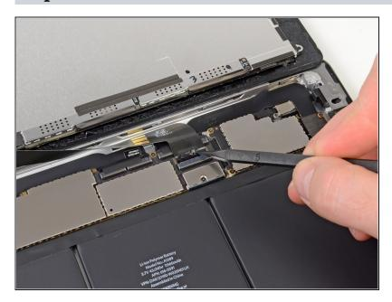
Using the tip of a spudger, peel back the piece of tape covering the LCD ribbon cable connector.
