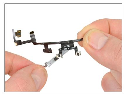
• Lift and remove the power & volume button ribbon cable.
