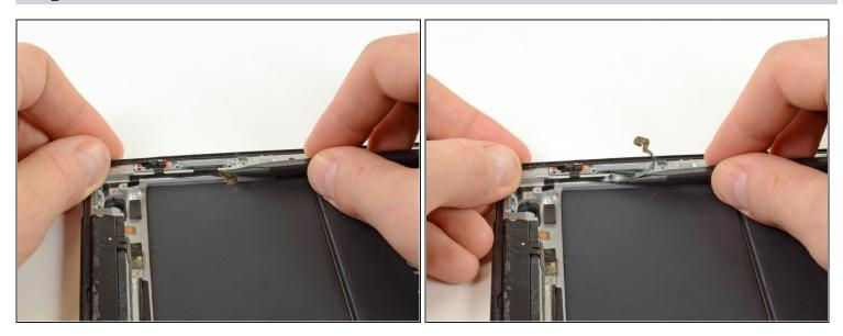
• Using the tip of the spudger rather that the wide edge, release the adhesive underneath the volume button branch of the ribbon cable.
