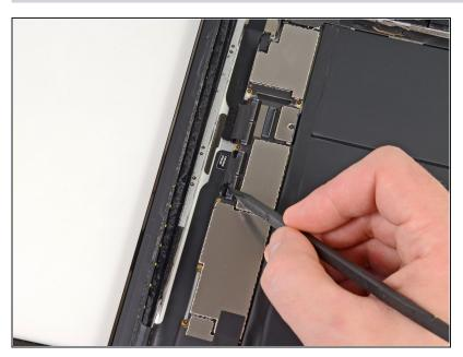
Using the tip of a spudger, peel back the piece of tape that secures the digitizer ribbon cable to the logic board.
