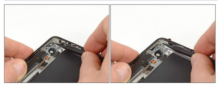
• With the tip of the spudger still underneath the ribbon cable, gently lift the power button out of its socket in the aluminum frame.
