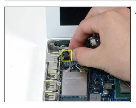
Disconnect the MagSafe board from the logic board.
