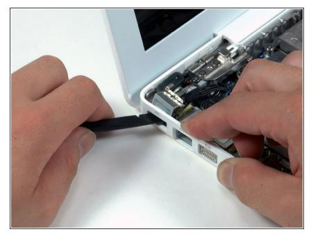
Use a spudger to rotate the MagSafe board up and out of its housing. It may be helpful to pull the lower case out slightly to provide additional clearance.
