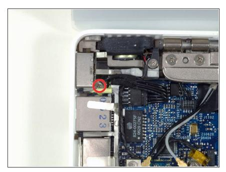
Remove the single Phillips screw securing the MagSafe board to the lower case.
