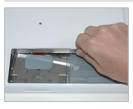
Lift up on L-shaped memory cover, slide it to the right, and lift it out of the computer.
