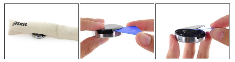
• The adhesive in the Moto 360 is proving to be a real challenge, so we heat. We heat again. And finally, we heat some more.
