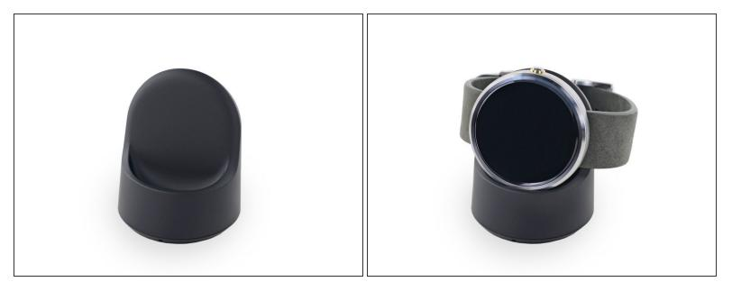
The Moto 360 is the first Android Wear smartwatch to ditch physical charging ports in favor of inductive charging.
