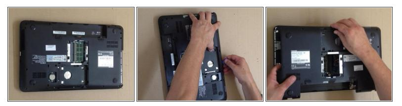
• Use a plastic tool for separating the bottom case from the laptop.
