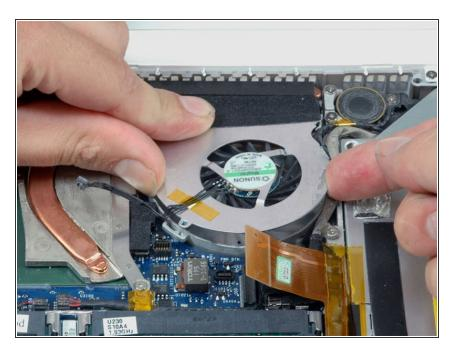
Push down on the left side of the fan and slide it slightly to the right in order to free the fan from the indicated tab on its right side. You can also use the tip of a spudger to free the tab on the right side of the fan.
