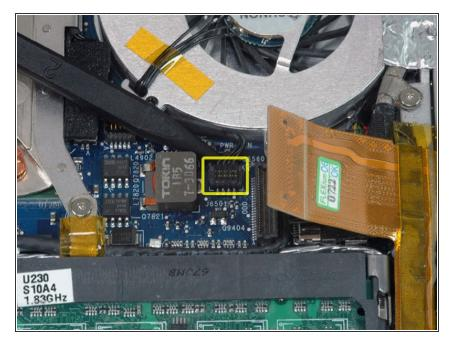
Use a spudger to disconnect the black fan connector from the logic board.
