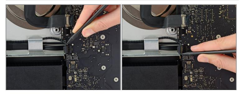
• Push on each side of the left speaker cable connector with the tip of a spudger and gently *walk* it out of its socket.
