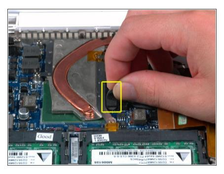
Peel up the small black rubber cover from the right side of the heat sink.
