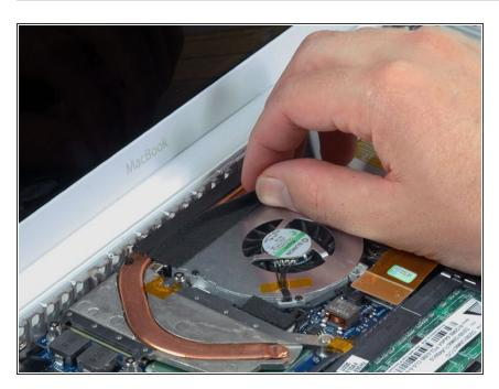
Carefully peel up the black felt tape between the heat sink and fan.
