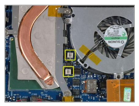
Disconnect the two newly-revealed temperature sensor connectors from the logic board.
