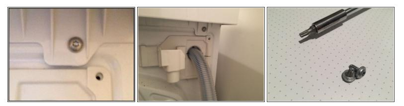
• To check the cable that might have come loose, we need to remove the top-lid (think before you act: this may void any guarantee by Siemens!). There are two screws at the back of the machine that need to be removed to be able to move the top-lid to the back and lift it.
