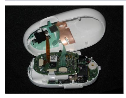
⚠ Carefully separate the two halves; do not pull on the flex cables.
