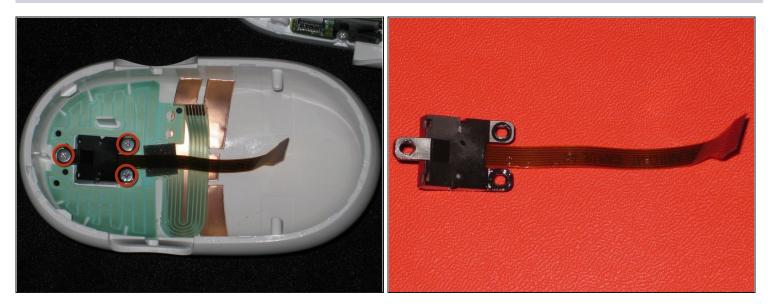
• Remove three Phillips #00 screws that attach the scrollball assembly to the upper shell.
