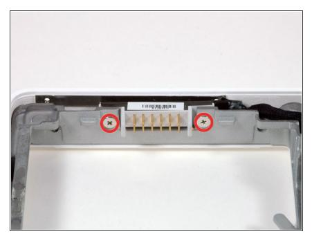
Remove the two Phillips screws attaching the battery connector to the lower case.
