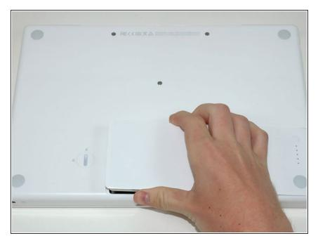
Lift the battery out of the computer.
