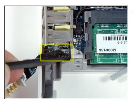
Use a spudger to carefully pry the battery connector up and disconnect it from the logic board.
