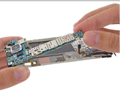
Let's jump right in to the belly of the beast. With the midframe halves separated, only a few connectors and a single screw hold the motherboard in place.
