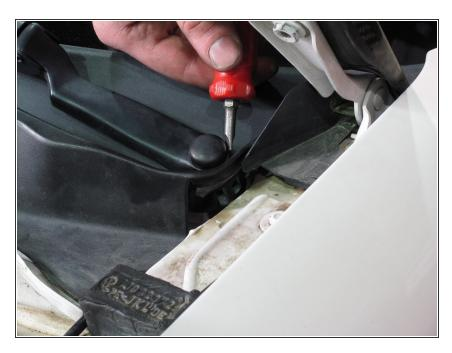
Use a flathead screwdriver to remove the cap from the windshield wiper.
