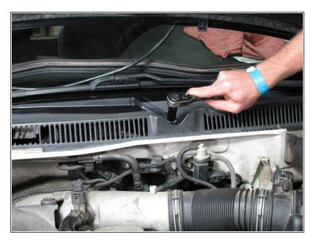
Use a socket wrench to release the passenger-side windshield wiper locking nut.
