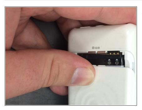
Slide off the back cover to reveal the battery.
