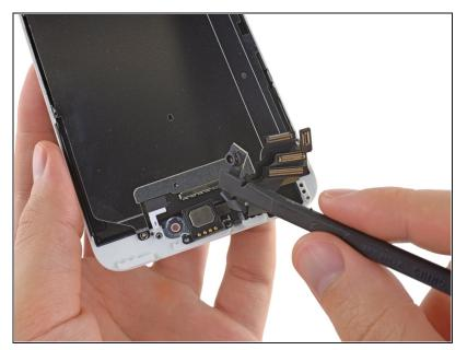
Use a the flat end of a spudger to pry up the front-facing camera and display cables, and gently push them aside.
