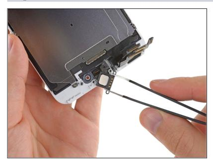
Use a pair of <u>tweezers</u> to firmly grasp and remove the earpiece speaker from the display assembly.
