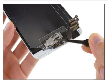
Lift and remove the earpiece bracket from the display assembly.
