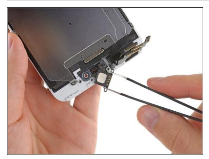
Use a pair of tweezers to firmly grasp and remove the earpiece speaker from the display assembly.
