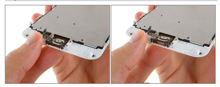
$\triangle$  The rubber gasket surrounding the home button is very thin and tears easily.
