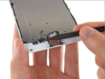
• Carefully use the tip of a spudger to finish separating the home button from the front panel.
