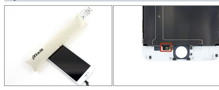
(i) The next step requires peeling one end of the home button cable (highlighted in red in the second picture) that is affixed to the back of the display assembly with strong adhesive. We highly recommend <u>using an iOpener</u> to heat the bottom of the display assembly, directly on top of the home button.
