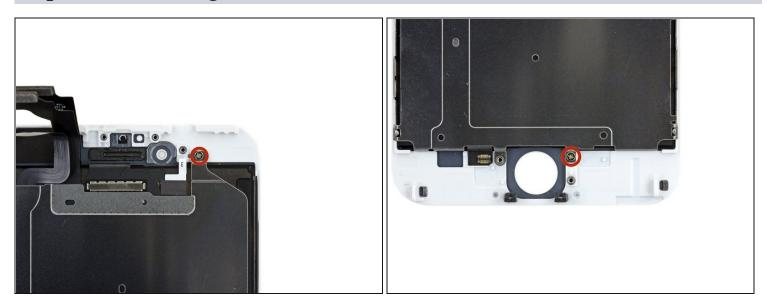
• Remove the two 1.7 mm Phillips screws (one on top and one on bottom) securing the LCD shield plate to the display assembly.
