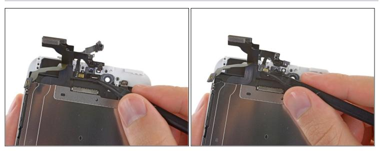
Pry the microphone portion of the front-facing camera and sensor cables from the display assembly.
