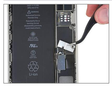
Remove the metal battery connector bracket from the iPhone.
