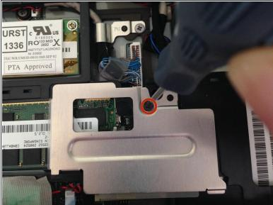
Using a #00 phillips head screwdriver, remove the 6mm screw holding the metal plate down.
