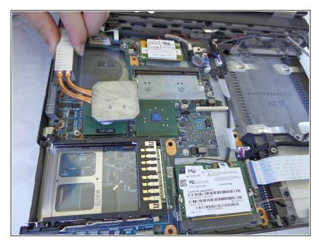
Wiggle the heat sink until it lifts off the top of your CPU. There is thermal paste underneath and it may stick.
