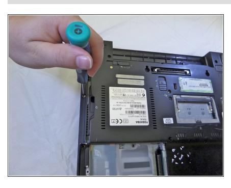
Remove the 4.5mm screw located under the CD-RW/DVD-ROM drive compartment, using a #00 phillips head screwdriver.
