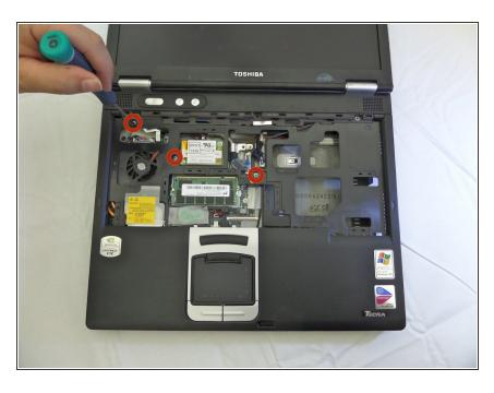
Using a #00 phillips head screwdriver, remove the three 13mm screws holding down the touch pad's frame from underneath the keyboard.
