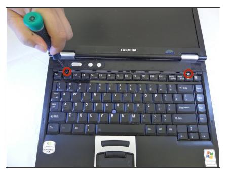
Using a #00 phillips head screwdriver, remove the two 4mm screws found underneath the keyboard strip.
