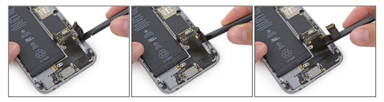
• Use the flat end of a spudger to begin peeling the Lightning connector assembly up from the rear case.
