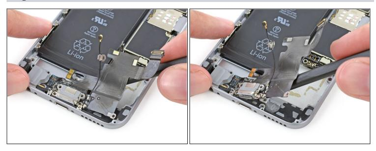
• Use the flat end of a spudger to lift under the Lightning connector portion of the assembly to free more adhesive.
