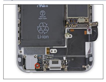
• Remove the single 3.6 mm Phillips #00 shoulder screw from the microphone brace.
