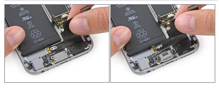
• Carefully pull the Lightning connector assembly up slightly to free it from the vibrator and speaker screw posts.
