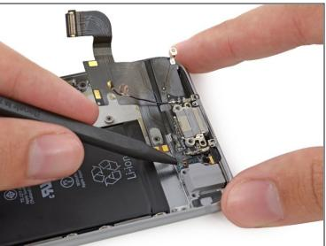
• Gently run the point of a spudger under the assembly between the Lightning connector and the headphone jack to free it from the last of the adhesive.
