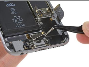
• Remove the Lightning port retaining bracket.
