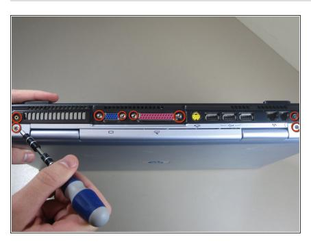
Remove eight screws from the back panel of the laptop.
