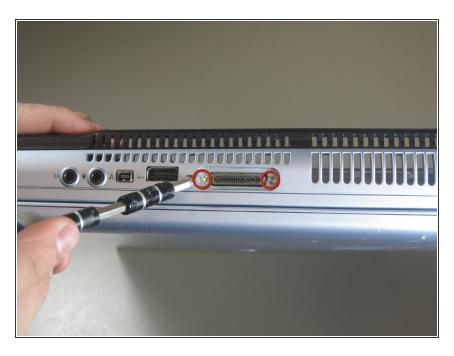
Using a flathead screwdriver, remove two screws on the left-side panel of the laptop.
