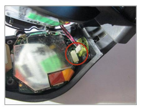
Pull the battery wires out from the motherboard slowly.
