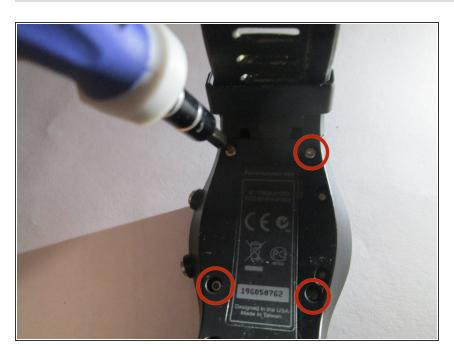
Unscrew the four 6.35 mm Torx T5 screws securing the backing of the watch.
