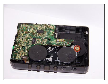
Replace the band, ensuring that it wraps around both large plastic revolvers and the small metal one.
