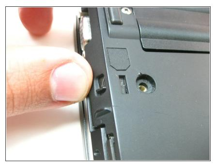
Push the small slider to unlock position, a tab will automatically pop out.
