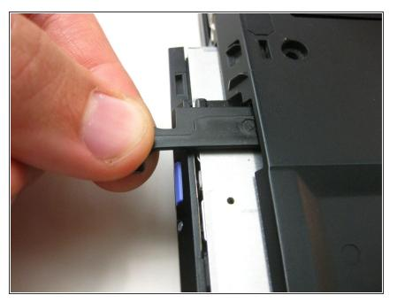
Pull the tab to dislodge the optical drive, then carefully pull the drive out.
