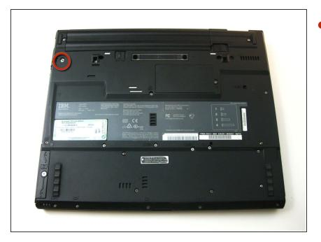
Remove the single screw holding the optical drive on the underside of the laptop
