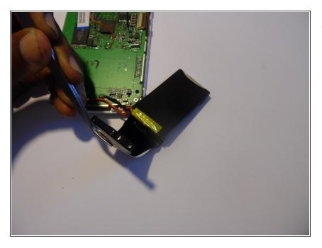
Unwrap the old battery from electrical tape and replace with new battery.
