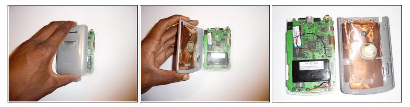
• Remove the back cover from the device exposing the battery.
