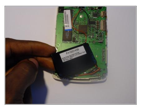
• Carefully remove the battery from the motherboard.
