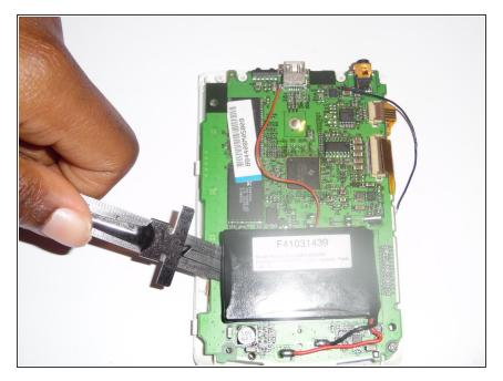
Using a plastic opening tool, small flathead screwdriver, or small knife blade pry the battery away from the motherboard. Be careful not to pry to fast, or you could rip the wires off during this stage.
