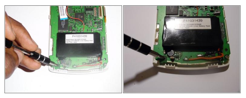
• Remove the two screws located at the bottom of the mothership, using a Philips head screwdriver.
