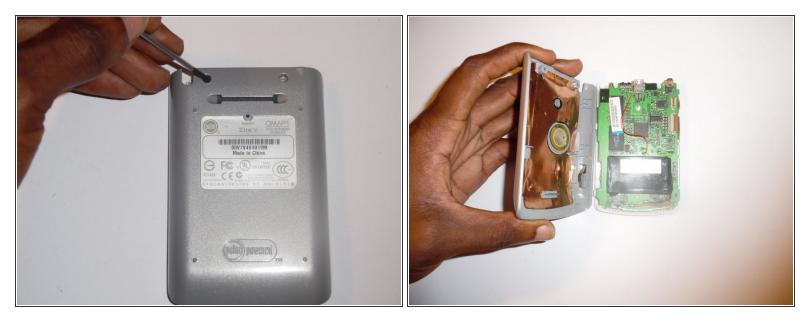
• Remove the two 0.8 mm screws located on the back of the device.
