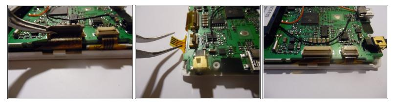
• Using tweezers, or something similar flip up the tab, releasing the wires located under the flap.
