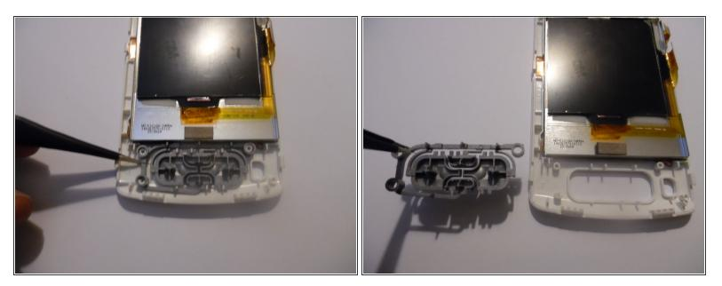
Using tweezers, or something similar remove the keypad from the device and replace with a new one.
