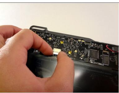
Once you see an even white line of the plastic pin casing appear (about 1 mm), use your index finger and thumb to pull the connector straight out from the motherboard.
