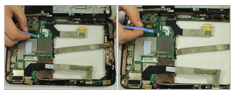
• Use the plastic opening tool to open the latch holding the last wire to the back of the device.
