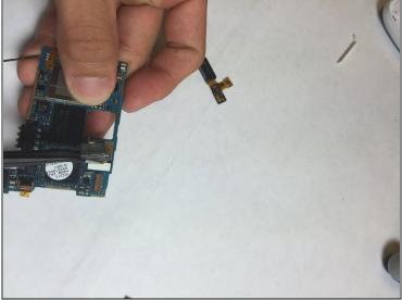
• Using tweezers pull out the back camera lens from the circuit board.
