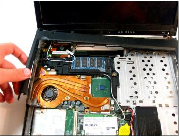
Remove the plastic bezel along the edges, you may need to pry the areas circled with a spudger to remove the bezel.
