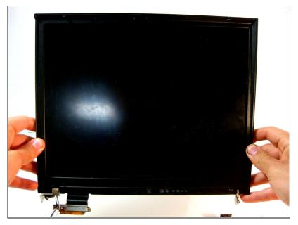
Carefully unplug the display ribbon on the motherboard, then carefully lift the display free from the device.
