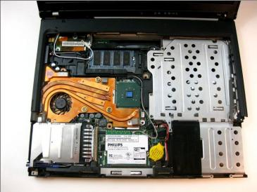
• Carefully maneuver the palm rest away from the keyboard, as both the keyboard and palm rest/trackpad will come off together.
