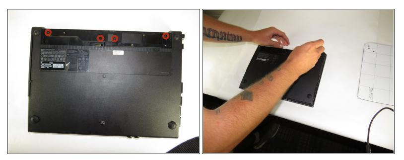
Unscrew the four (2.5 mm Phillips) screws (Use Phillips #0 Screwdriver).
