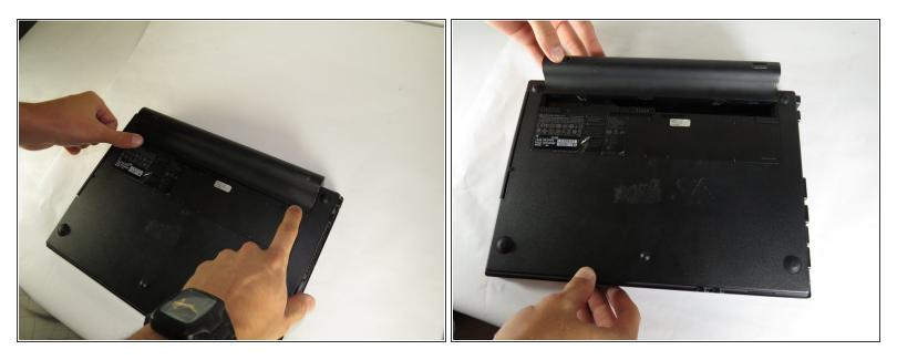
• Flip the laptop upside down and remove battery by pressing inward on the two latches holding the battery in.
