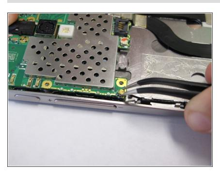
Use tweezers to unplug the sub cables from the circuit board and housing.
