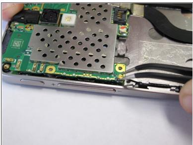
Plug in new sub cables to the circuit board and housing.
