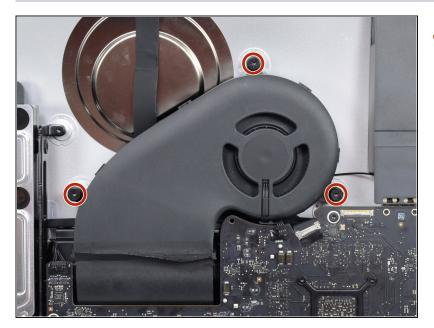
Use a T10 Torx screwdriver to remove the three 12.4 mm screws securing the fan.
