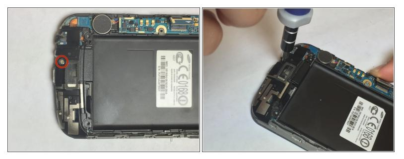
• Unscrew 4.4mm with a PH #000 marked screw.
