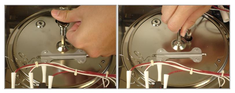
• Remove rod from the center of the plate with a wrench.
