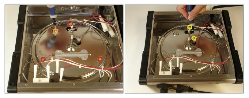
• Remove screws #1 Phillips screwdriver bit.
