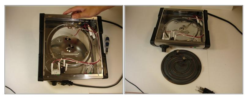
Remove plate carefully as to not damage internal components i.e. insulator, metal frame, wires, etc.
