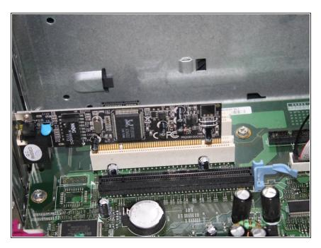
With your free hand, gently squeeze the sides of the card. Pull upwards to release it from the tab slots that hold it in place.
