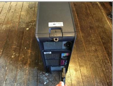
Power down your PC and remove the power cord from the back.
