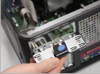
Gently push the release tab on the card retention latch from the inside to pivot the latch open. The latch will remain in the open position
