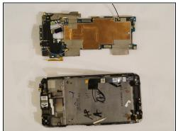
• Completely remove the motherboard.
