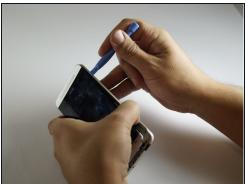
Gently remove the volume button. Using a plastic opening tool or guitar pick, loosen the back panel of the phone. Work around the phone, following the crease of the back panel.
