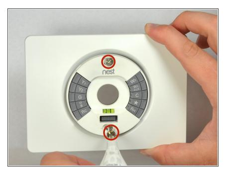
Remove the two 40mm screws from the base of the thermostat using a #0 Phillips screw driver.
