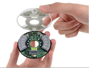
Pry the base mother board open from the side using a plastic opening tool.
