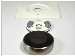
Unsnap the base from the trim plate (if used) using a plastic opening tool.
