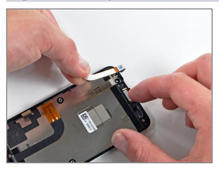
Gently lift the front-facing camera out of its recess in the inner case and remove it from the Evo.
