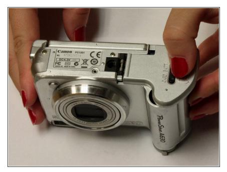
Slide the tab on the battery door while pushing the battery door out from the camera.
