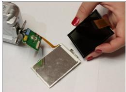
Use a spudger to gently remove the LCD screen from the metal backing plate
