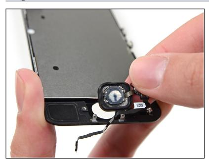
Remove the home button assembly from the front panel.
